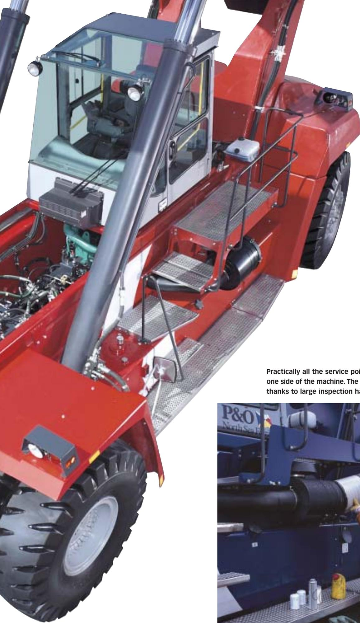
Practically all the service points are easily accessible on one side of the machine. The drive line is easily accessible thanks to large inspection hatches.
