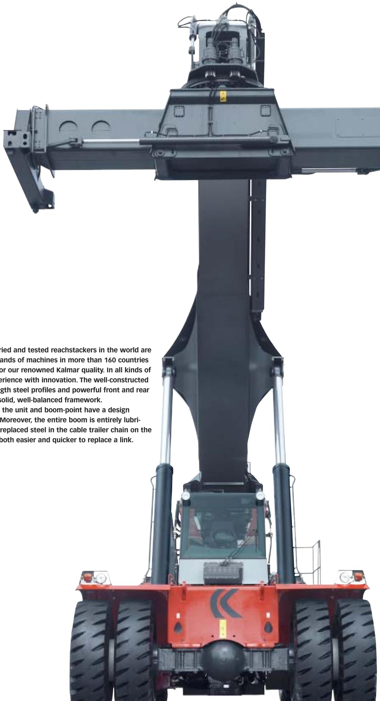
The most extensively tried and tested reachstackers in the world are made by Kalmar. Thousands of machines in more than 160 countries have made us known for our renowned Kalmar quality. In all kinds of areas we combine experience with innovation. The well-constructed chassis with high-strength steel profiles and powerful front and rear cross-heads provide a solid, well-balanced framework.
