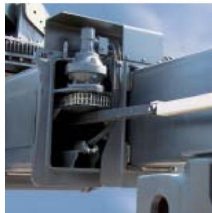
Chains have replaced cylinders to control the outreach from 20 to 40 feet. The unit reaches out more evenly and with greater precision. Loading and unloading are quicker.
