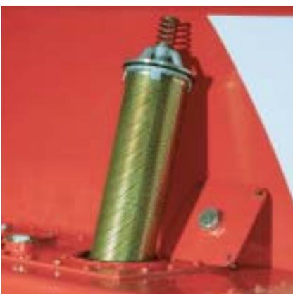
Return filters for the hydraulic oil come as standard, maintaining cleaner oil and reducing wear on hydraulic components. One of many details that help assure longer service intervals.
