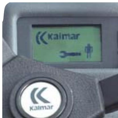
The driver or service personnel obtain a rapid diagnosis on the display, eliminating the need for time-consuming fault finding via measurements from one connection point to the next.
