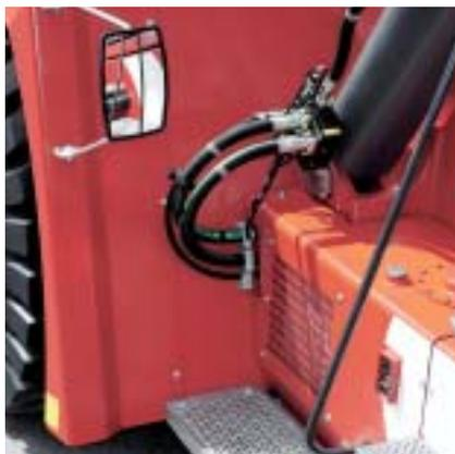
Previously separate units are built together in fewer blocks. All hydraulic pipes have been replaced by hoses, thus reducing the number of couplings. The hoses are also thicker, leading to lower pressure falls and less heat.
