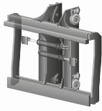
Carriage sideshift / fork positioning
