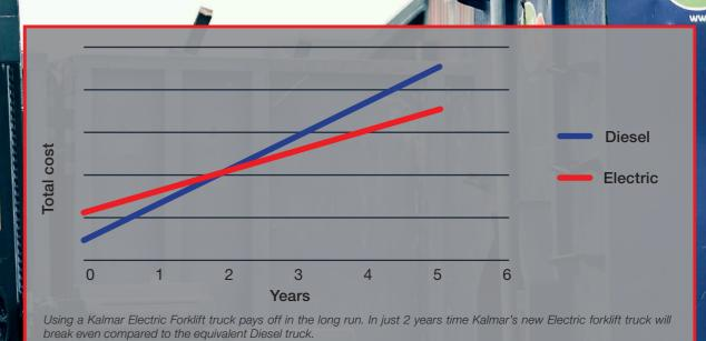
Note: Calculations are based on 2,500 operational hours per year, a diesel consumption of 8 litres/h at 1.2 €/litre,
